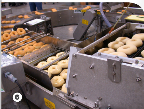
Above: 4– Standard Mark VI system 5– Mark VI system with automatic Proofer and Glazer 6– Automatic proofer with Deep Mark VI fryer in Automatic system
