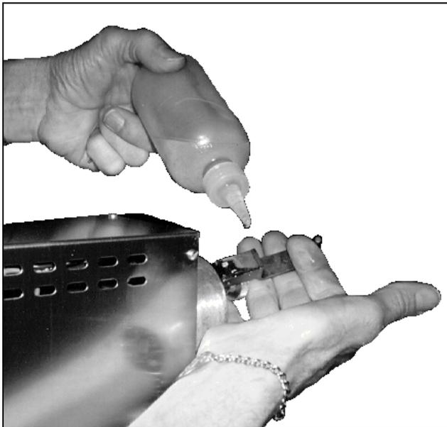
Figure 2-1. Lubricating the Connecting Rod.
