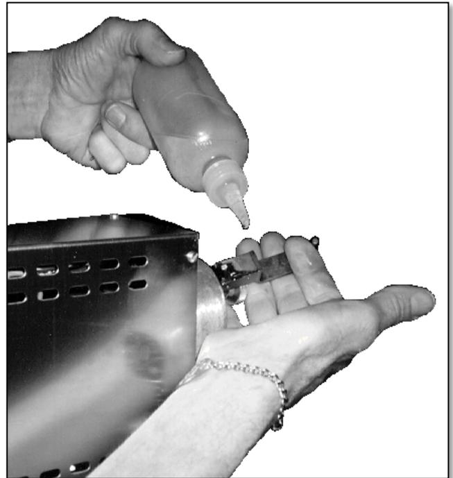
Figure 6 Lubricating the Connecting Rod.
